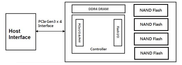
Figure 2-1 Functional Block Diagram
