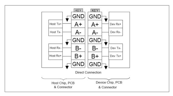
Figure 3-2 Direct Connection between the Host and Device
