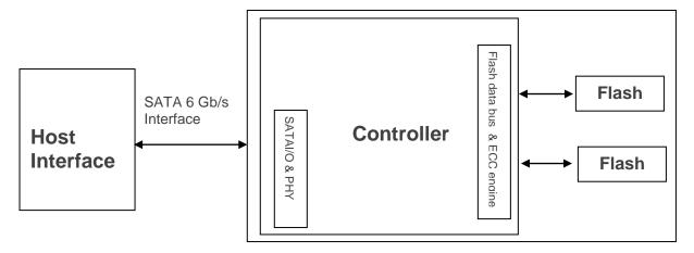
Figure 2-1 Block Diagram
