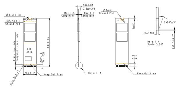
Figure 10-2 Dimensions - Double Side
