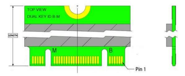
**Figure 3-1 Pin Connectors**
