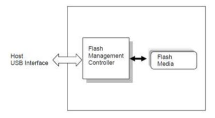
Figure 2-1 Functional Block Diagram
