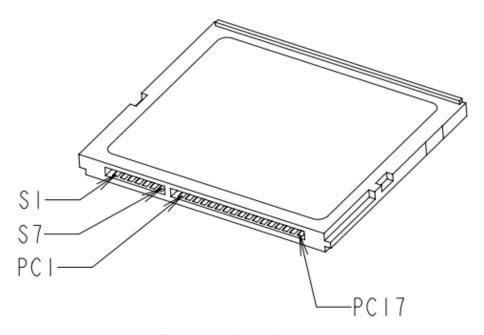
Figure 3-1 Pin Assignment
