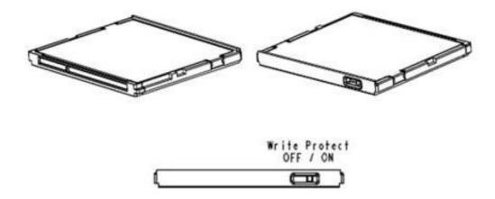
Figure 9-2 Write Protect Switch
