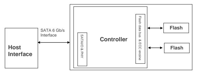
Figure 2-1 Functional Block Diagram
