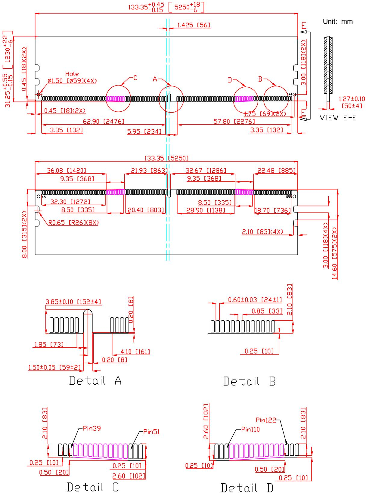
(All dimensions are in millimeters with  $\pm 0.15$ mm tolerance unless specified otherwise.)
