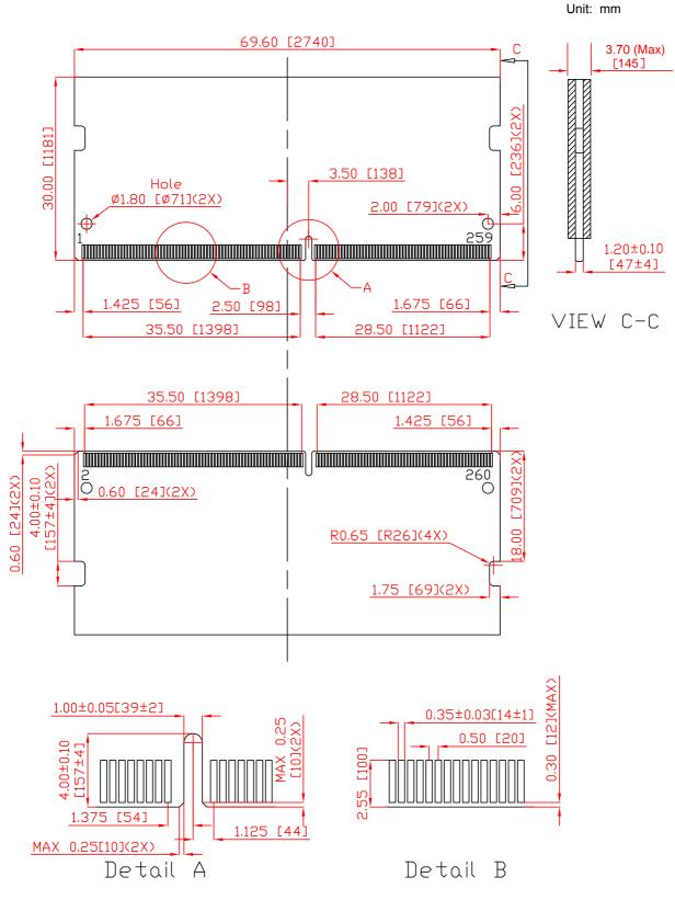
(All dimensions are in millimeters with ±0.15mm tolerance unless specified therwise.)
