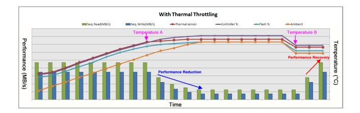
When the temperature exceeds the threshold value, the drive starts to throttle by decreasing in performance by multiple stages, thereby allowing the device to cool down. It measures the temperature level again and, if it is greater than or equal to the previous reading, it goes one step further, reducing the performance by one more level until it reaches a low steady state.
