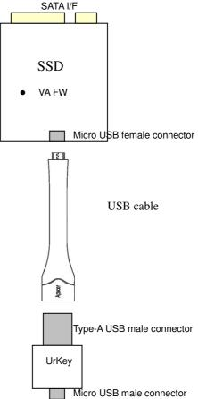
Operation wise, the UrKey can activate Erase, Destroy or Protect depending on customized requests. However, the methods to trigger may vary. For instance, to trigger Erase or Destroy, simply insert the UrKey and the corresponding feature will be executed automatically. The process will be performed continuously until it is completed, even if the UrKey is removed. In contrast, Write Protect is enabled when UrKey is unplugged. To use the SSD in normal status, plug the UrKey.
