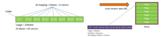
4K Page mapping uses one page as the unit of mapping. The most important characteristic of page mapping is that each logical page can be mapped to any physical page on the flash memory device. This mapping algorithm allows different size of data to be written to a block as if the data is written to a data pool and it does not need to take extra operations to process a write command. The below example shows how page-level mapping performs a write command:
